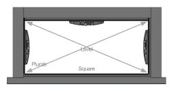
$3.\ensuremath{\,\text{To}}$  install bottom track, cut to length, then screw at 400mm centres, insure track is level, pack if needed.
