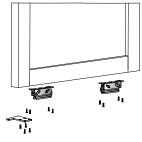
7. Pre Drill and CSK holes for 8g screws at 400mm centres, into top guide track.
