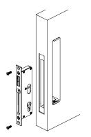
7. Insert Second handle Into frame, following steps 5 and 6 with the driving pin connecting into the Handle.
