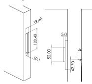
Please note: Dimensions for lock and handles have all clearance added and all dimensions are set to fit lock Easily.
