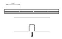
9. Fix interlocker with 8g screws.
