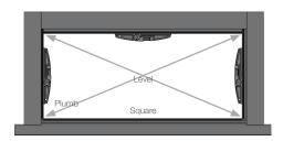
3. To install bottom track, cut to length, then screw at 400mm centres, insure track is level, pack if needed.
