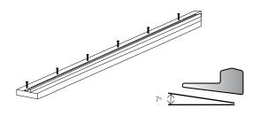
5. Screw rollers into bottom rail. Ensure adjustment screws are facing outwards. Fix negative load hook near end of door.
