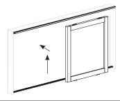
10. Use adjustment screws to make door run level with the top and bottom tracks. Take the weight off the door while adjusting.
